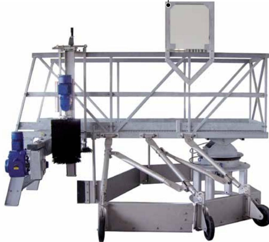
The wheel bearings are SKF quality bearings with bearing housings made from composite material. Gears are surface treated as standard according to type 3.1/EN 12944 cor. Cat. C3. Bogie is equipped with a rotation monitoring.
