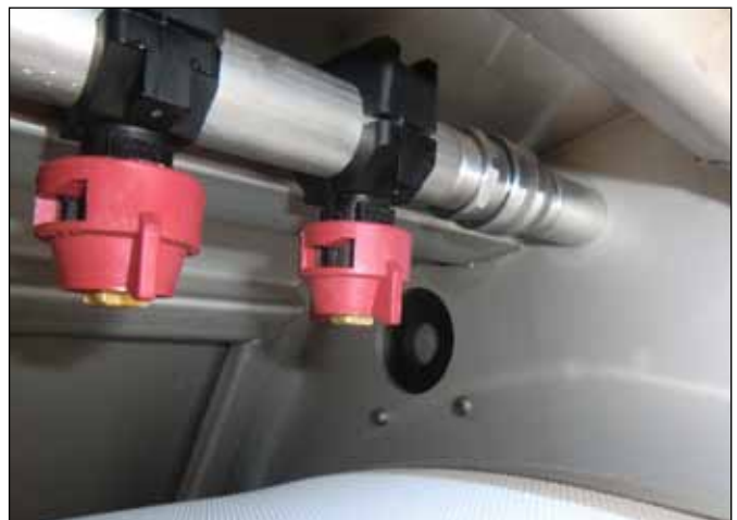
Flussing pipe with nozzles type click on and fast release joint.
