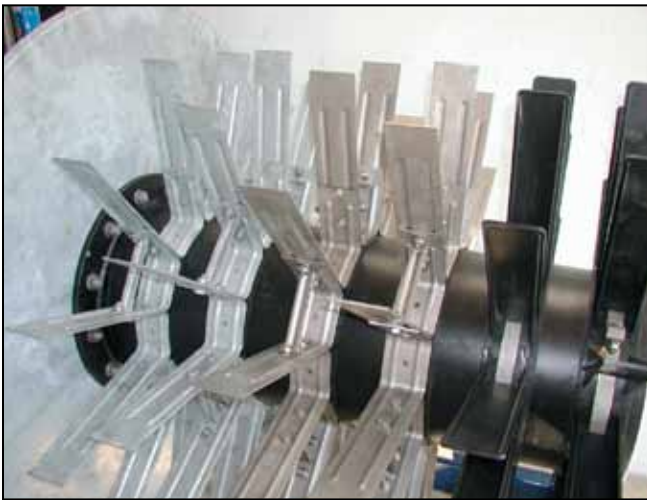
The above picture shows rotor blade material qualities. Shown from left to right are hot-galvanised – stainless steel (AISI304) – acid-resistant (AISI316) – and glass fibre reinforced plastic blades.
