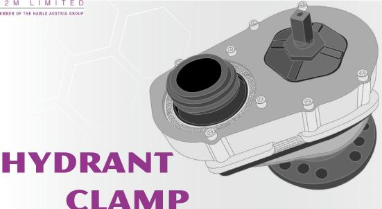
The **R2M HYDRANT CLAMP** is a high quality, easily installed single solution external fitting, designed to make safe a reported issue of corrosion and potential failure of the series 19 Hydrant inlet/outlet securing clip. This can lead to the risk of the outlet adapter and main chamber unscrewing during operation and fitment of external pressure pipe apparatus, causing a serious health and safety risk to operators.
